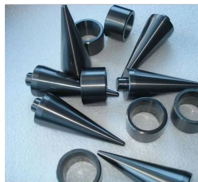
Carbide sleeves and cores after machining
