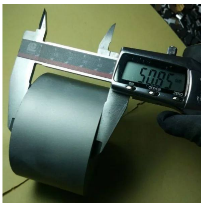
Carbide die blank under caliper check at 50.05 mm during inspection
