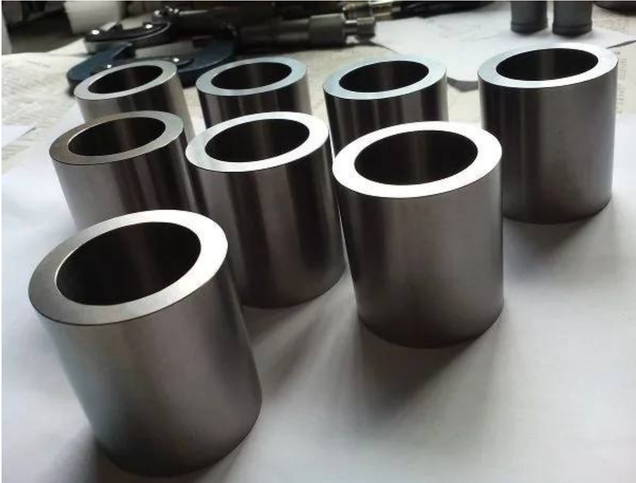
Tungsten carbide tubes and bushes after grinding of bore and outside diameter
