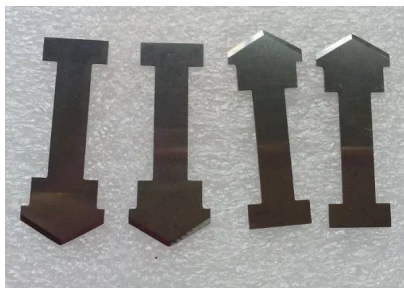
Carbide cutter blanks with brazing faces prepared
