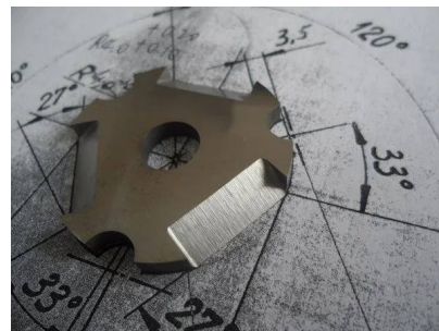
Profiled carbide cutter with central bore and indexed teeth
