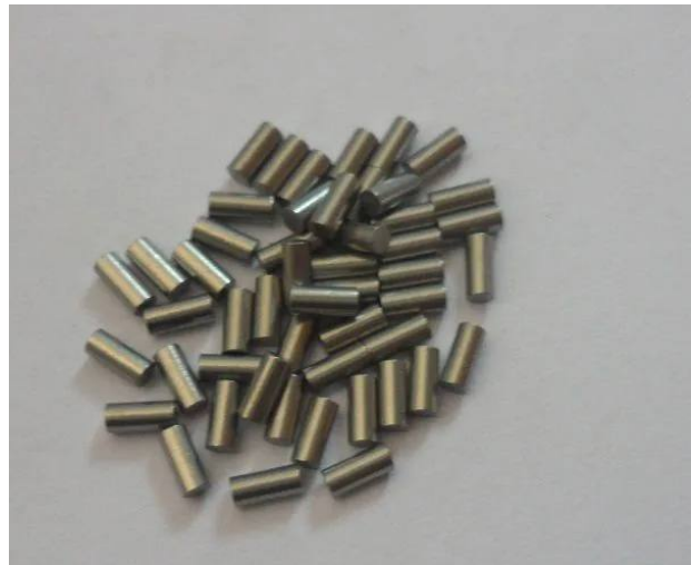
Carbide pin blanks after grinding ready for pressing into holders
