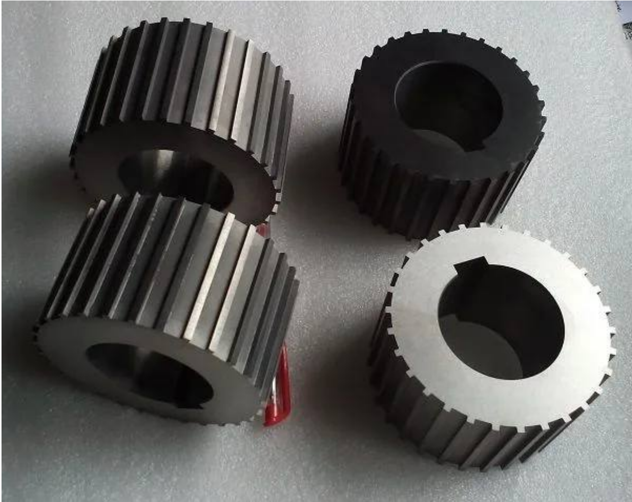
Tungsten carbide gear and matching toothed ring after profile machining
