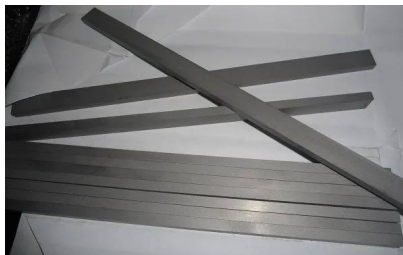
Carbide strips in several cross sections ready for despatch
