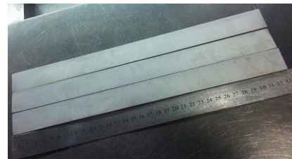
Long carbide strips prepared for wear plate and knife applications
