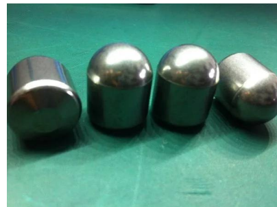
Ballistic and spherical carbide buttons after grinding
