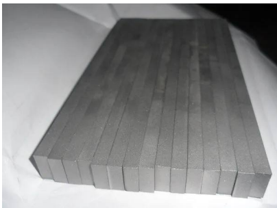
Stacked tungsten carbide strips after grinding
