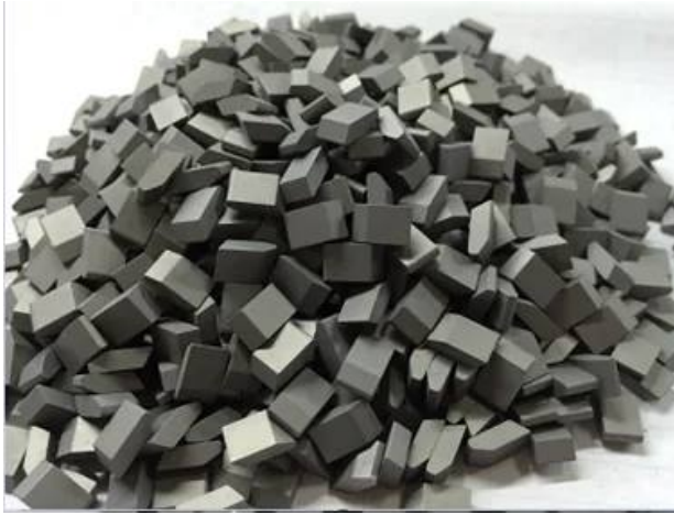
Tungsten carbide saw tips in production quantity ready for brazing
