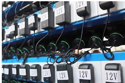
Aging rack running units to catch early failures
