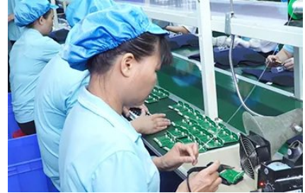
Control board soldering before boards enter a housing
